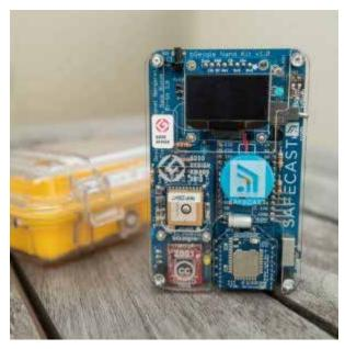
Figure 22: the bGeige Nano, a portable handheld Geiger counter that is widely used by Safecast volunteers<sup>80</sup> Source: <u>https://safecast.org/devices/</u>
